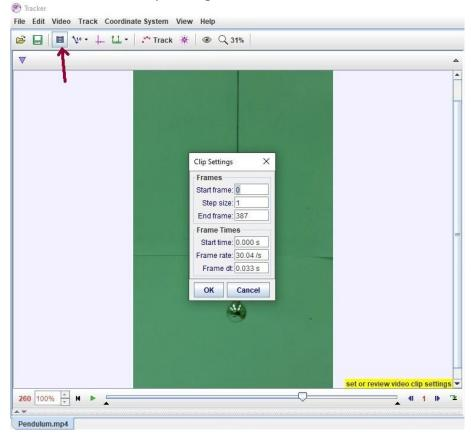
In frame 155 create a point mass on the bob and start automatic tracking [ Track - > New - > Point mass, then Ctrl+Shift+click on the bob, then Search At each frame where auto-tracking stops, select "Accept" ]
